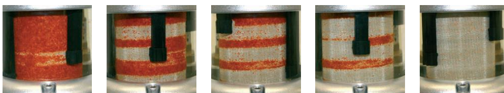
Offset Point of Rotation cleaning arms travelling around the mesh and sucking off the contaminants
